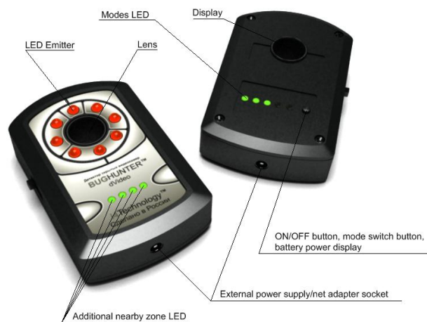
Picture 2 – main parts location
