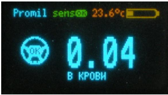
Picture 9 – test result in Ppm (blood alcohol content - the result is obtained by applying the relation: 1 ppm = 0.500 mg / l)
