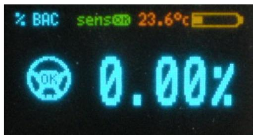
Picture 8 -test result in% BAC (blood alcohol content - result obtained by applying the ratio of 1% BAC = 0,05 mg / l)
