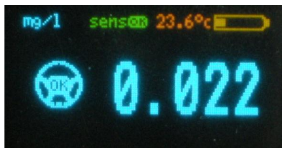
Picture 7 – test result in mg/l (of alcohol, contained in exhaled air)
