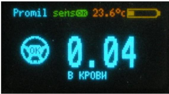
Picture 9 – test result in Ppm (blood alcohol content - the result is obtained by applying the relation: 1 ppm = 0.500 mg / l)
