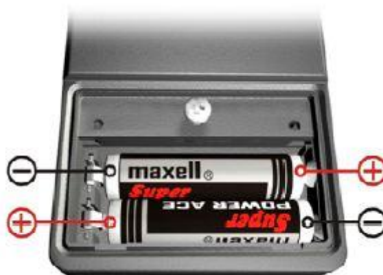
Picture 3 – Installation of batteries into the compartment
